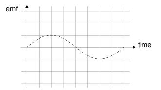
Which graph represents the induced emf produced when the same generator rotates 400 times in 40s? The original induced emf is shown by the dashed line.
